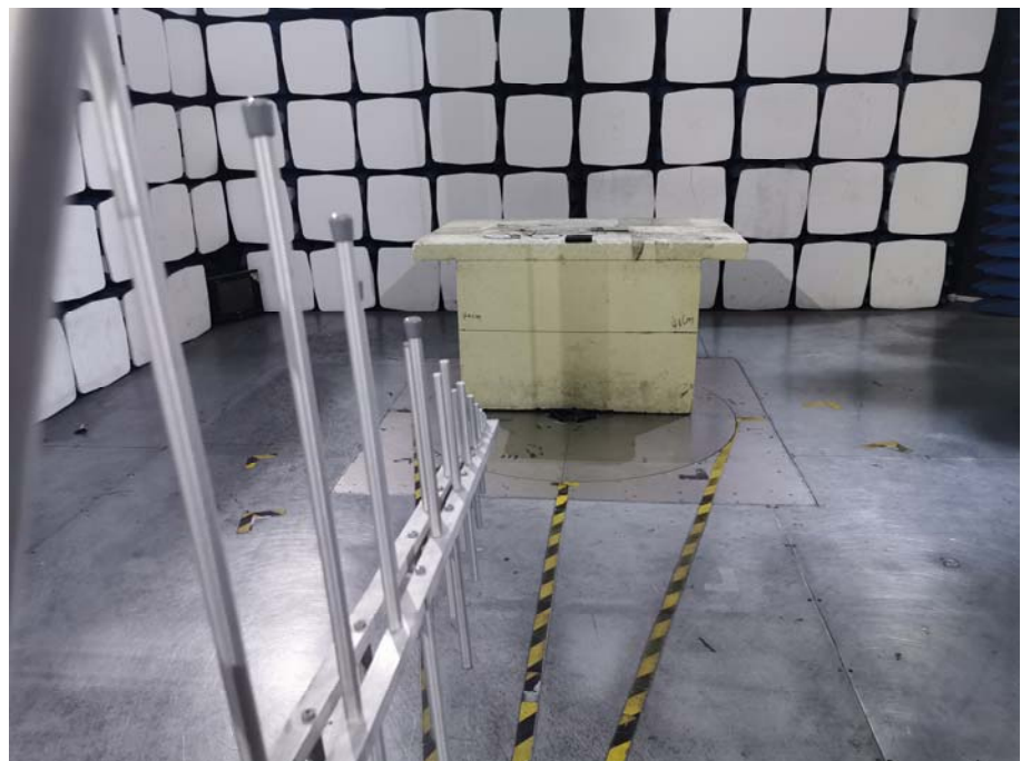
Radiation Emission Test Setup (30MHz to 1GHz)
