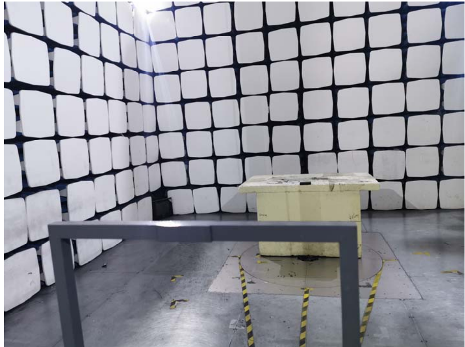
Radiation Emission Test Setup (Below 30MHz)
