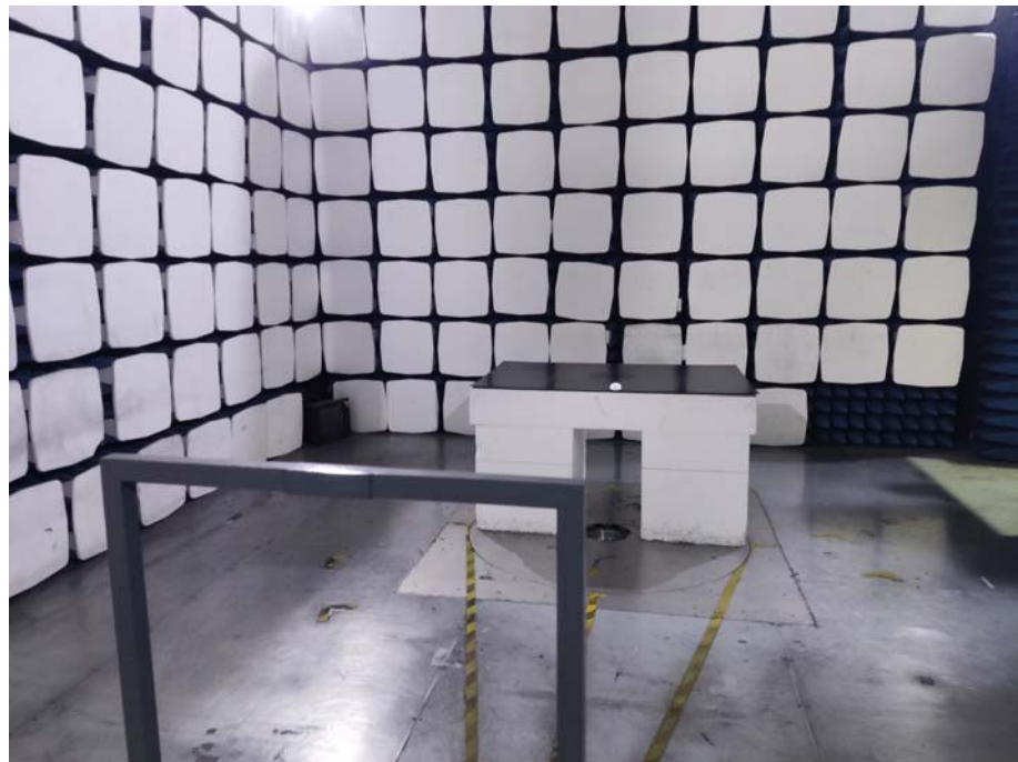
Radiation Emission Test Setup (Below 30MHz)
