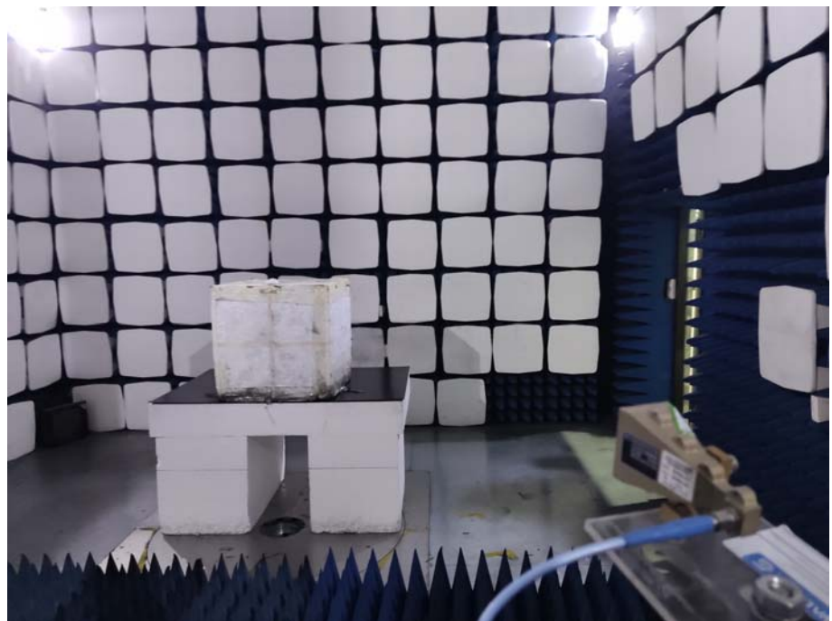
Radiation Emission Test Setup (Above 18GHz)
