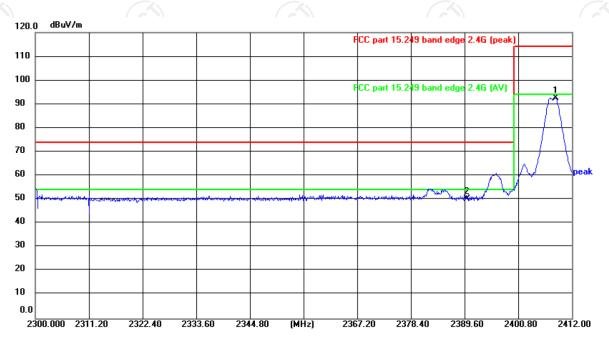
Site Polarization: Horizontal Temperature:  $24(^{\circ}\text{C})$  Limit: FCC part 15.249 band edge 2.4G (peak) Power: Humidity: 52%
