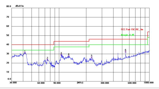
Site #2 3m Anechoic Chamber Polarization: Vertical Limit: FCC Part 15C RE\_3m Power:
