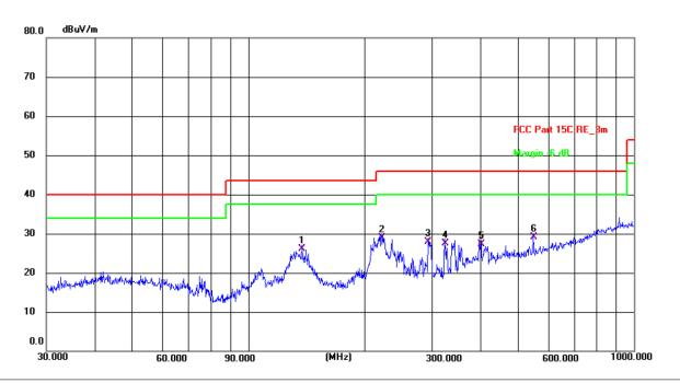
Site #2 3m Anechoic Chamber Limit: FCC Part 15C RE\_3m Polarization: Horizontal
