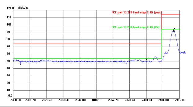
Site Polarization: Vertical Temperature:  $24(^{\circ}\text{C})$  Limit: FCC part 15.249 band edge 2.4G (peak) Power: Humidity: 52%
