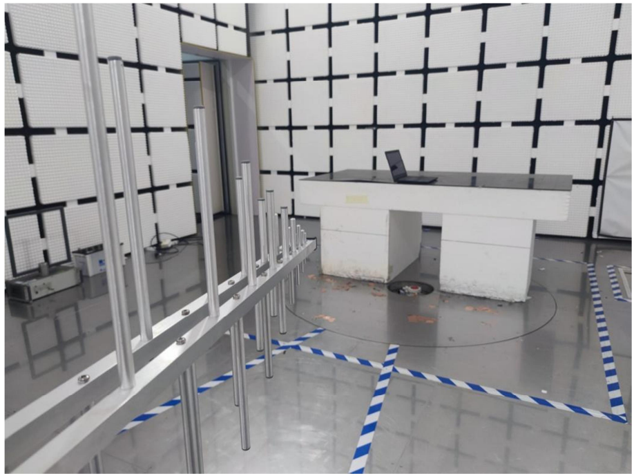
Radiation Emission Test Setup (30MHz to 1GHz)
