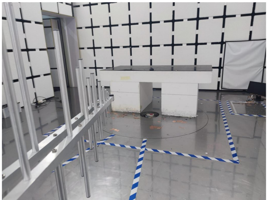
Radiation Emission Test Setup (30MHz to 1GHz)
