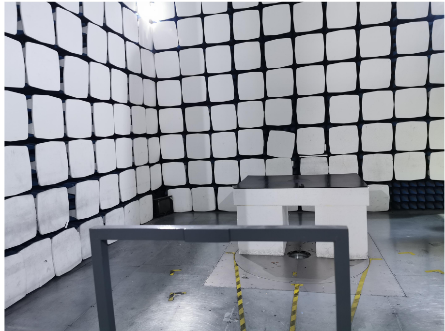
Radiation Emission Test Setup (Below 30MHz)
