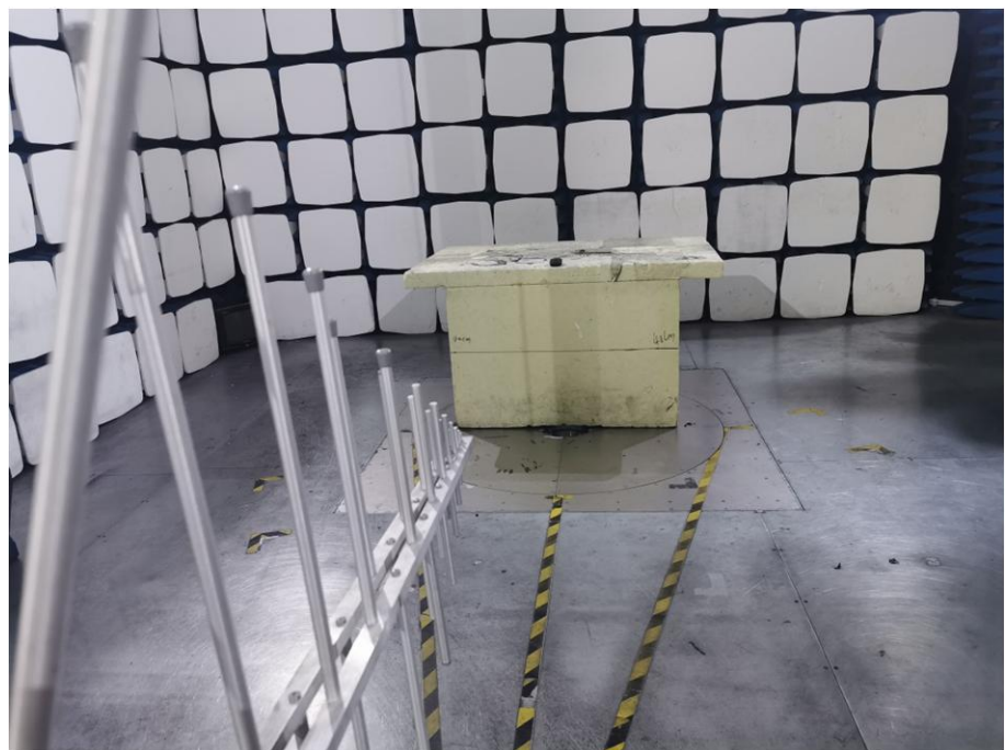
Radiation Emission Test Setup (30MHz to 1GHz)
