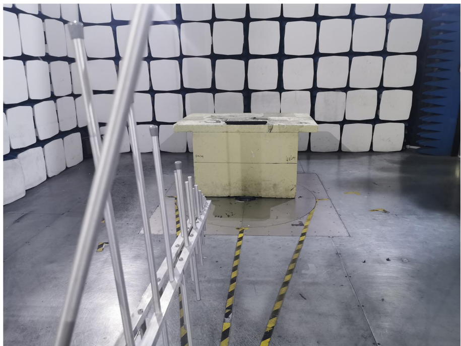
Radiation Emission Test Setup (30MHz to 1GHz)
