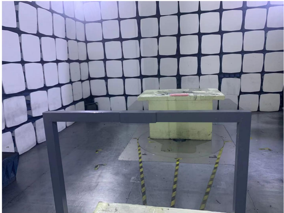
Radiation Emission Test Setup (Below 30MHz)
