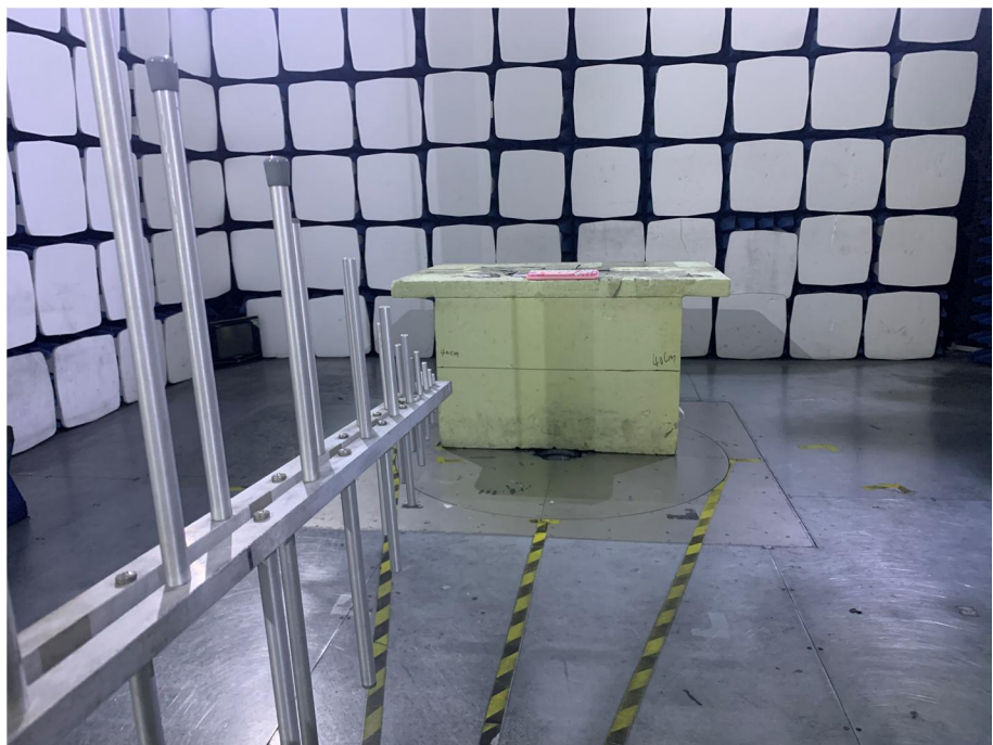
Radiation Emission Test Setup (30MHz to 1GHz)
