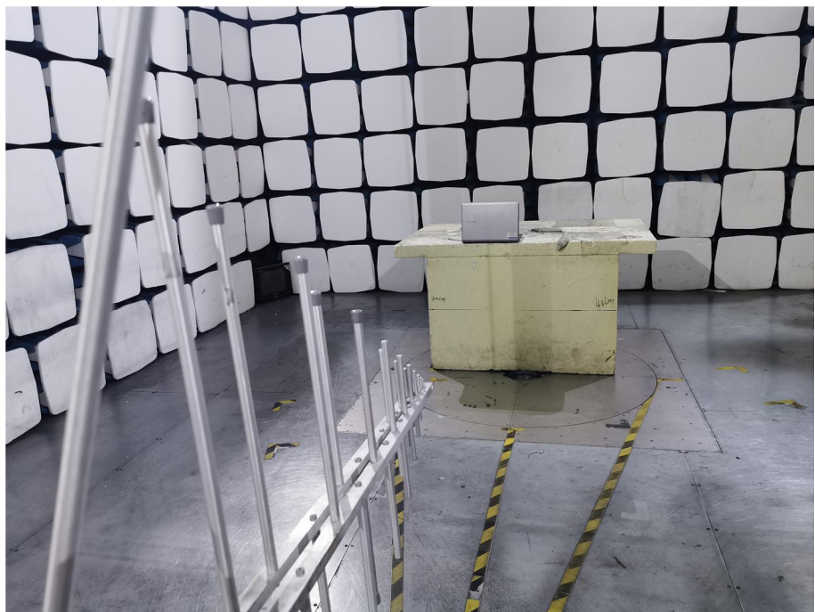
Radiation Emission Test Setup (30MHz to 1GHz)
