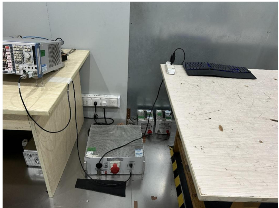
Conducted Emission Test Setup
