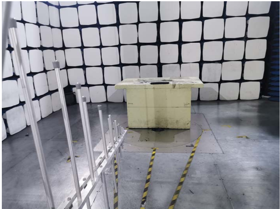
Radiation Emission Test Setup (30MHz to 1GHz)
