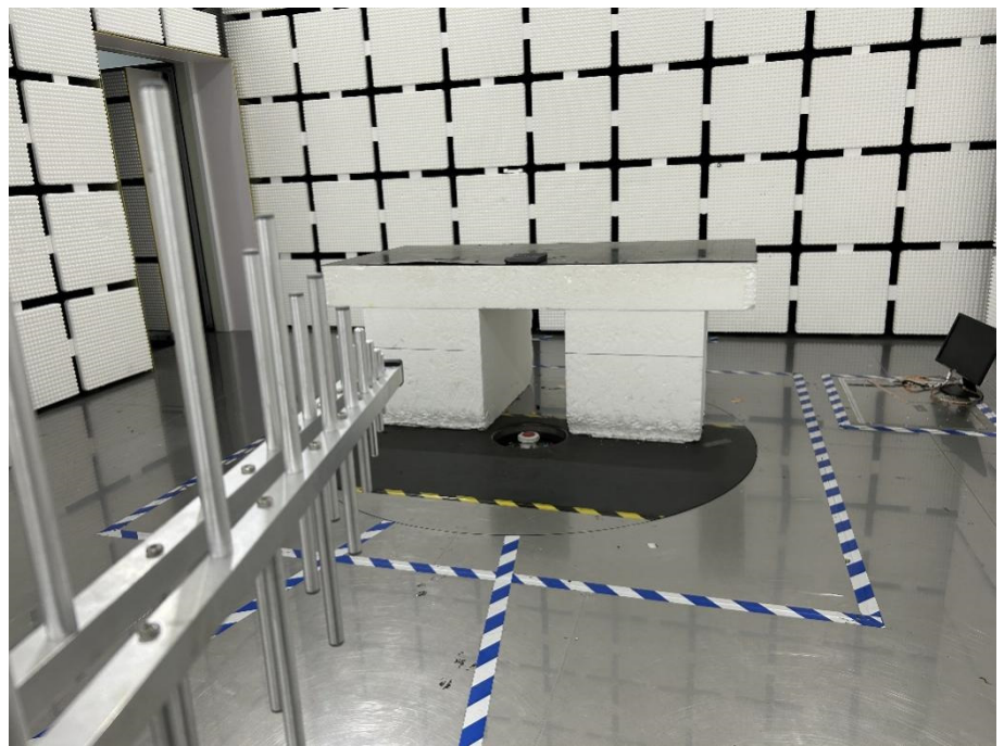
Radiation Emission Test Setup (30MHz to 1GHz)
