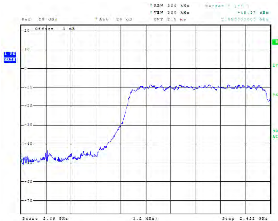
Figure 120 Plot of Low Band Edge Compliance (40MHz N Mode, 2422 MHz, Chain 1)
