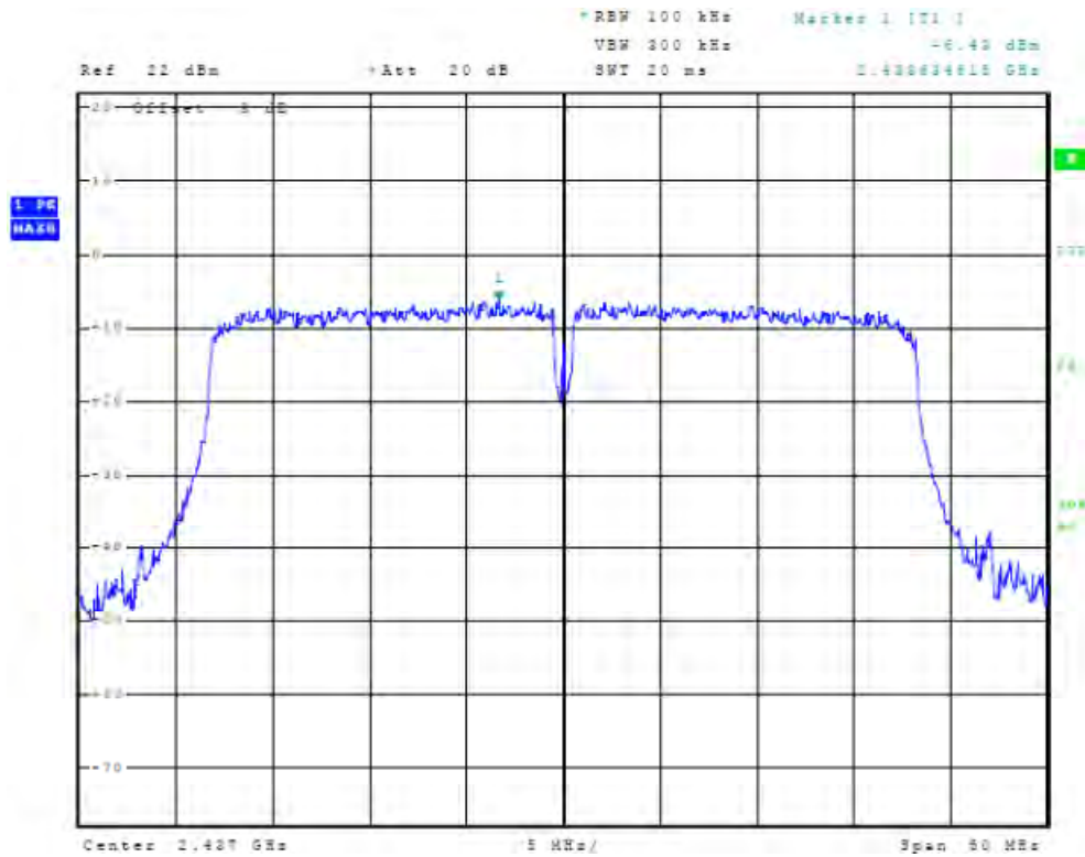
Figure 91 Plot of Power Spectral Density (40 MHz N Mode, 2437 MHz, Chain 1)
