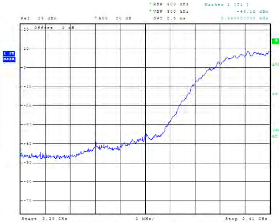
Figure 111 Plot of Low Band Edge Compliance (20MHz CCK Mode, 2412 MHz, Chain 0)
