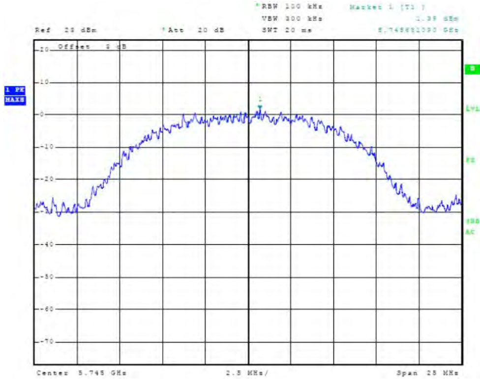
Figure 93 Plot of Power Spectral Density (20 MHz CCK Mode, 5745 MHz, Chain 0)
