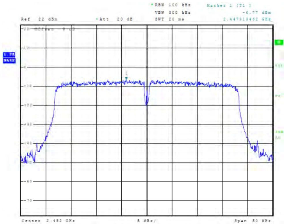
Figure 92 Plot of Power Spectral Density (40 MHz N Mode, 2452 MHz, Chain 1)
