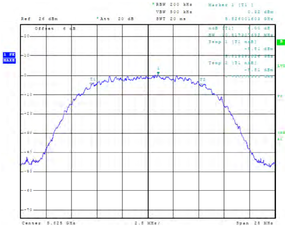
Figure 59 Plot of 6dB Band width (20 MHz CCK Mode, 5825 MHz, Chain 0)
