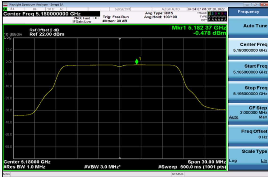
**Power Spectral Density Data Plot (CH Mid)**
