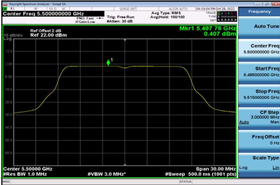
**Power Spectral Density Data Plot (CH Mid)**
