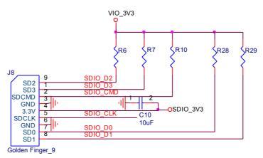
Figure 2. WiFi verification connection interface to Host SDIO
