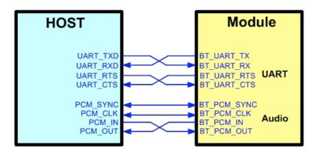
Figure 3. Bluetooth verification connection interface to Host UART
