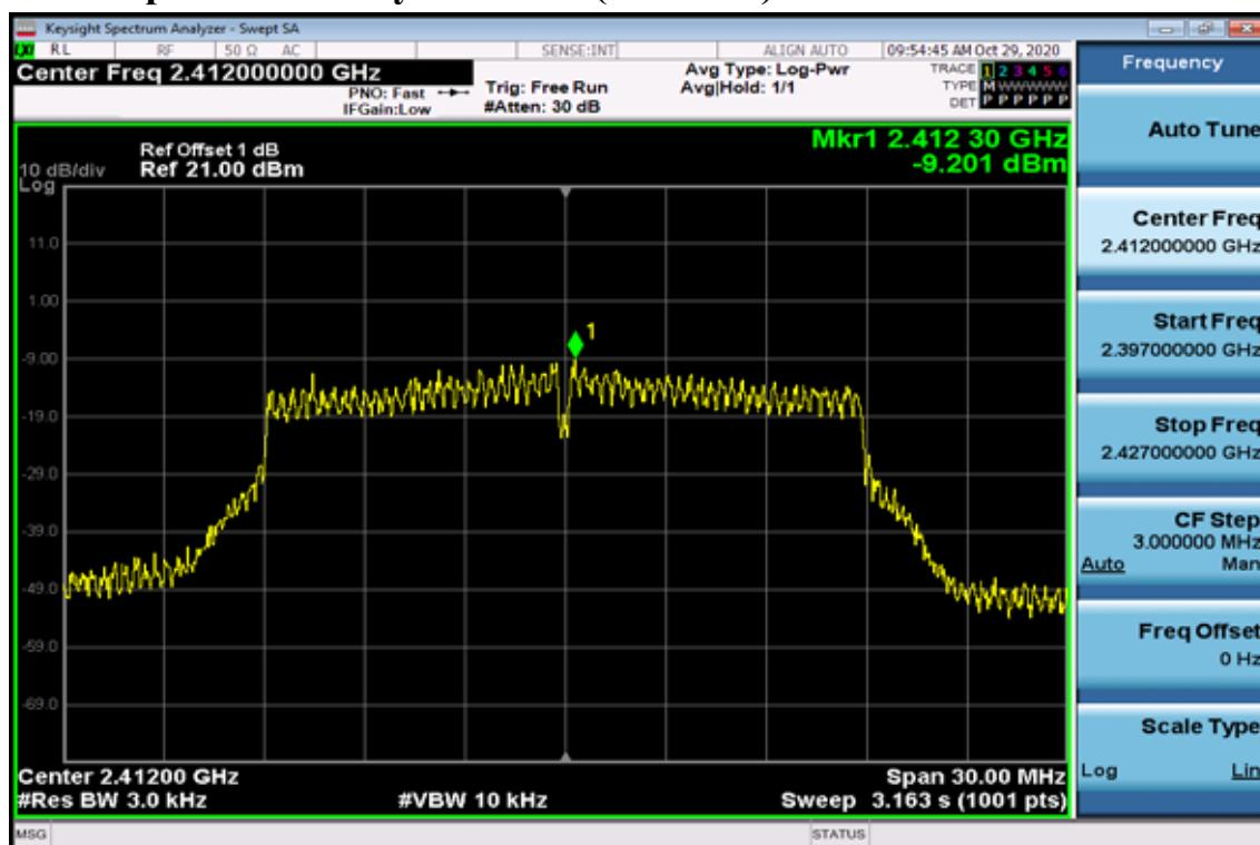
**Power Spectral Density Test Plot (CH-Mid)**
