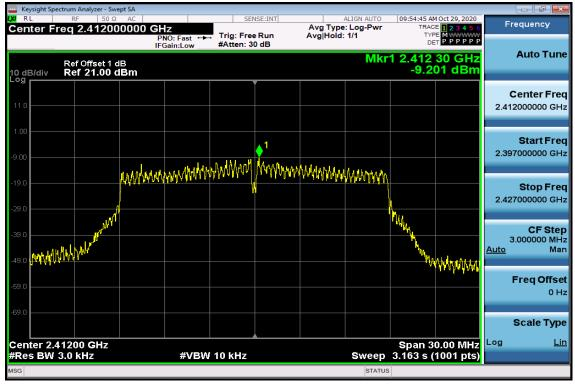
Power Spectral Density Test Plot (CH-Mid)
