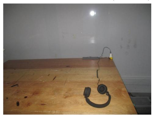
2. Radiated Emissions (30MHz-1GHz) Test Setup
