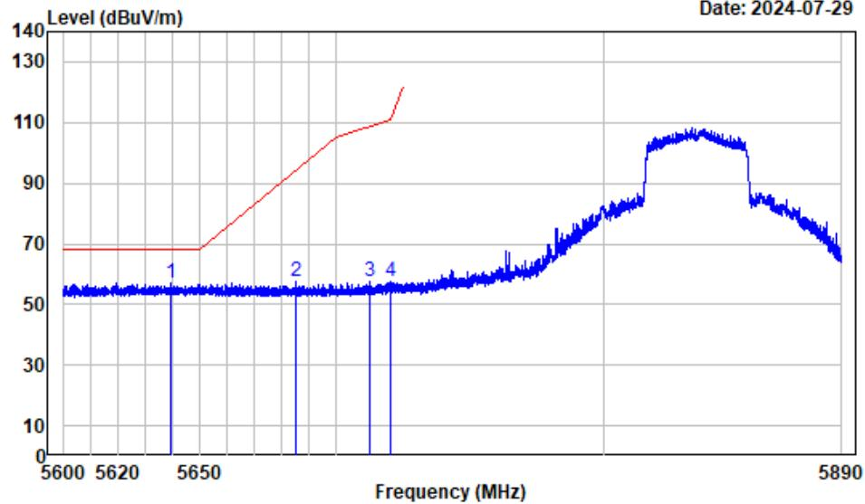
**802.11ax-HE40**Test Channel: **5835MHz** Ant. Polar. : **Vertical**
