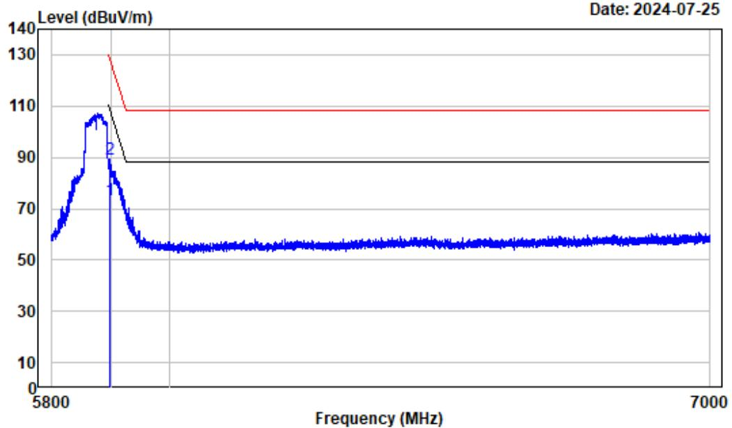
**802.11ac-VHT80**Test Channel: **5855MHz** Ant. Polar. : **Horizontal**
