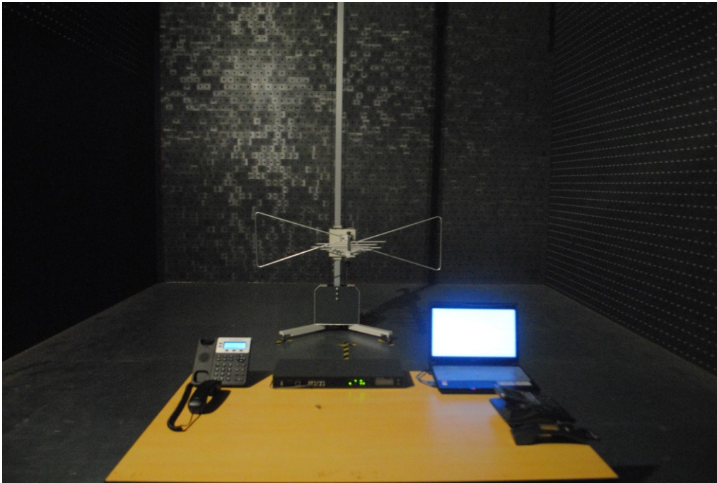
Radiated Emission test view (Frequency above 1GHz)
