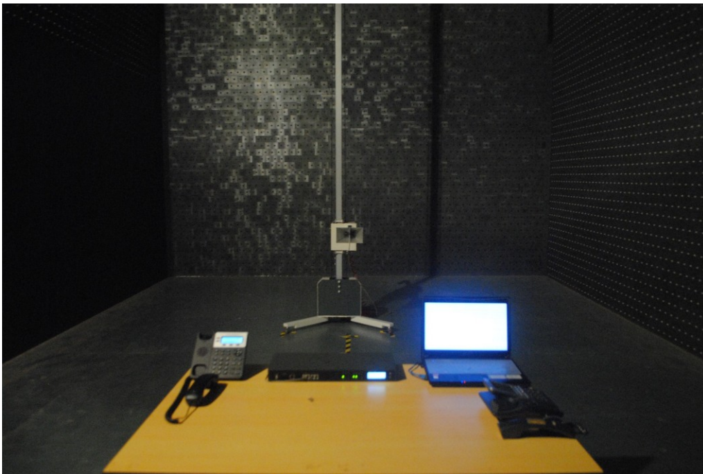
Radiated Emission test view (Frequency above 1GHz)
