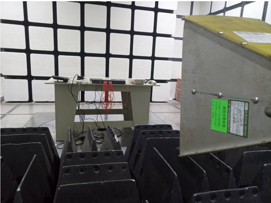
Radiated Emissions – Rear View (Above 1 GHz)
