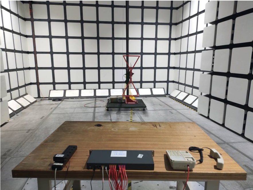
Radiated Emissions – Rear View (Below 1 GHz)
