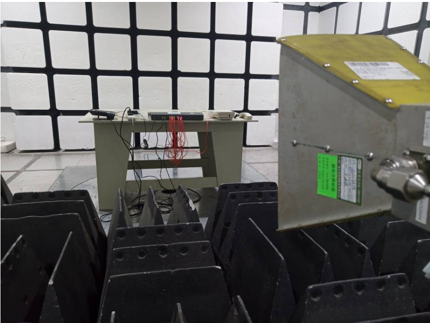
Radiated Emissions – Rear View (Above 1 GHz)
