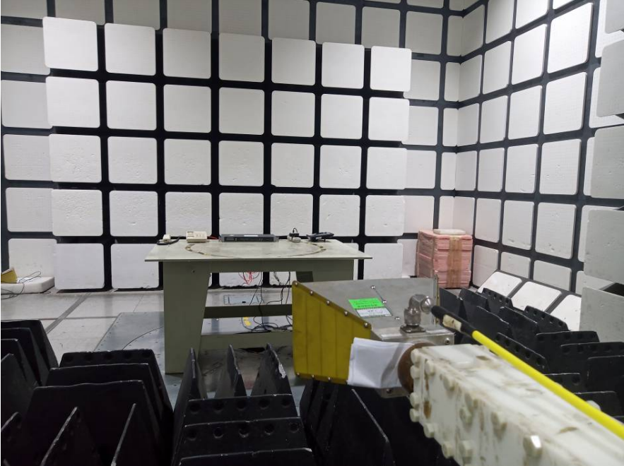
Radiated Emissions – Front View (Above 1 GHz)
