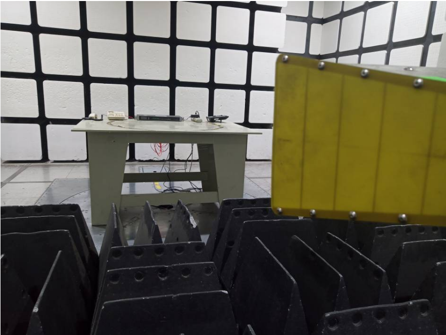
Radiated Emissions – Front View (Above 1 GHz)
