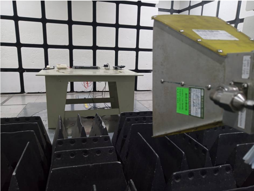
Radiated Emissions – Front View (Above 1 GHz)
