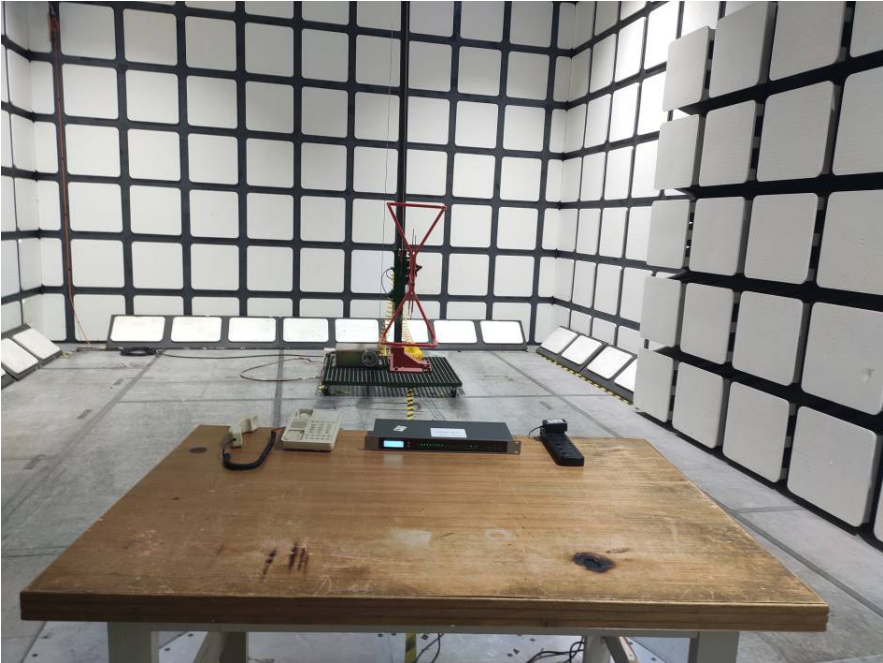
Radiated Emissions – Front View (Below 1 GHz)
