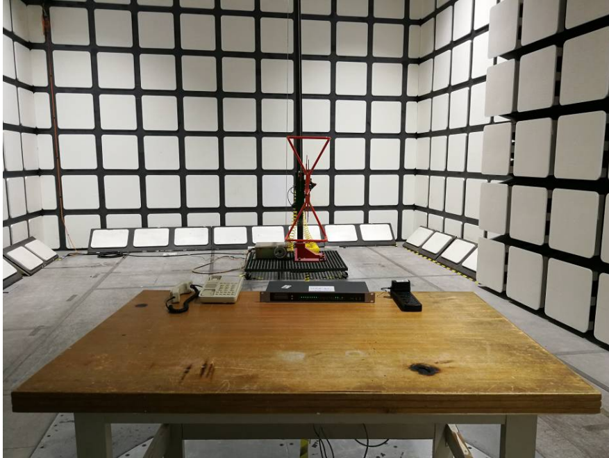
Radiated Emissions – Front View (Below 1 GHz)
