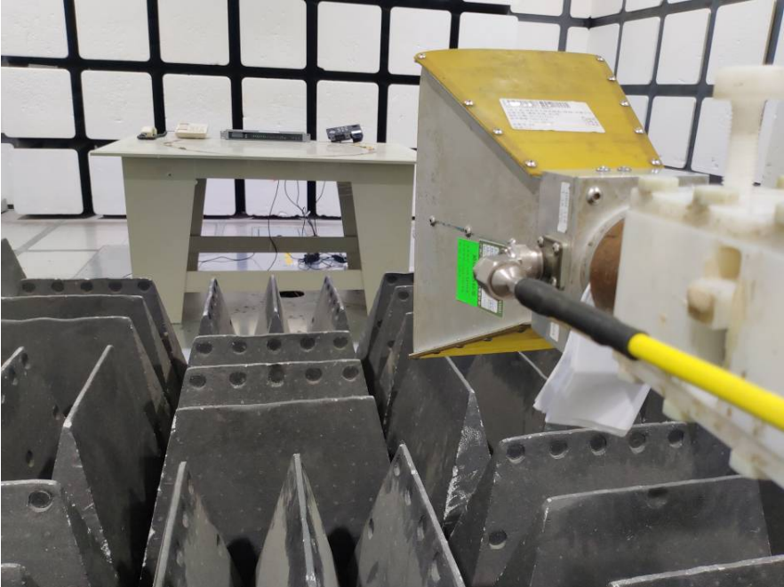
Radiated Emissions – Front View (Above 1 GHz)
