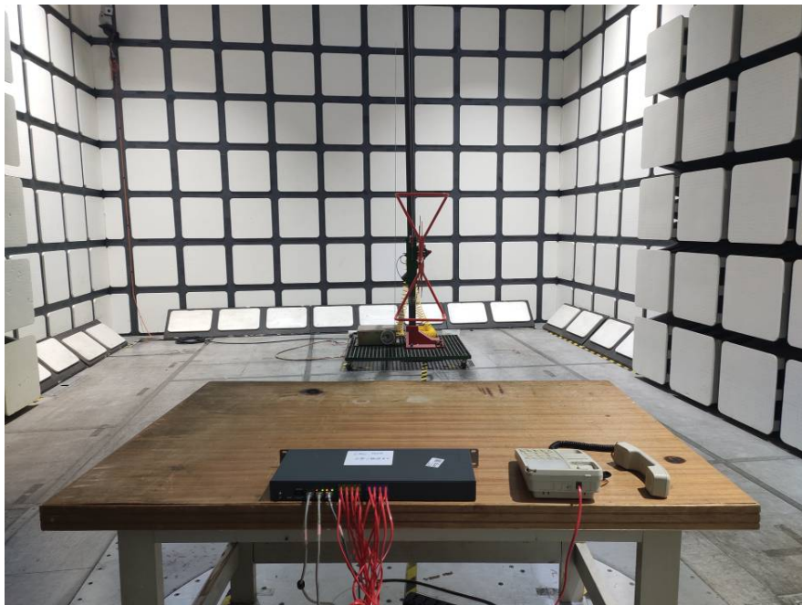
Radiated Emissions – Rear View (Below 1 GHz)
