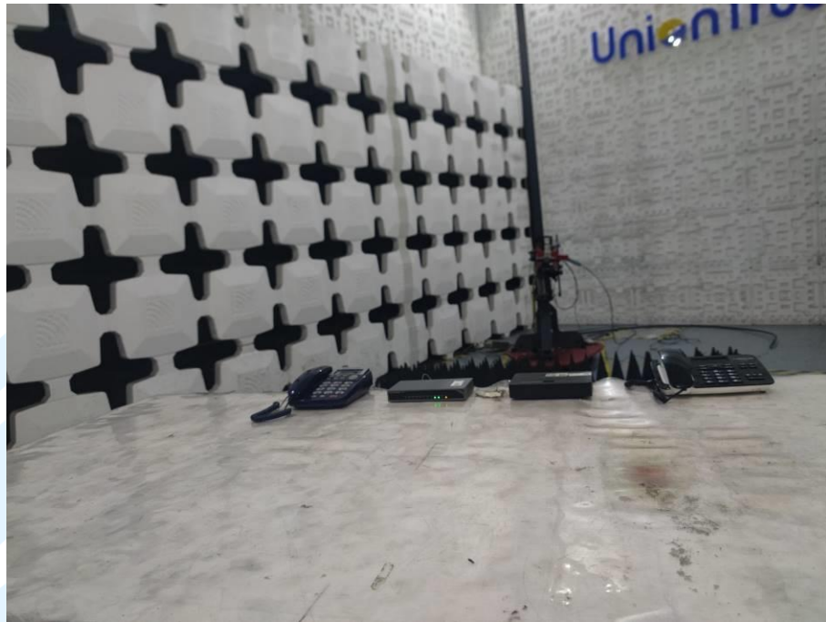
Radiated Emission Test Setup-2 (Above 1 GHz)
