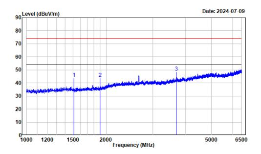
Site : chamber B Condition : Vertical Project Number: 2401U56421E-EM Test Mode : Communication+ Adapter (A907-120100W-US2) Tester : Dylan
