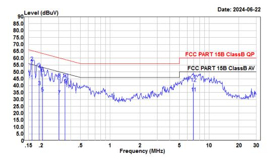
Condition: Neutral Project : 2401U56421E-EM test Mode: Communication+ Adapter (GQ12-120100-AU) tester : Macy.shi
