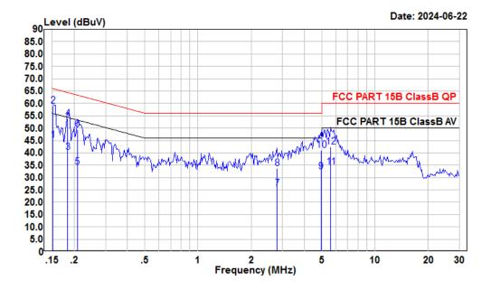
Condition: Neutral Project : 2401U56421E-EM test Mode: Communication+ Adapter (DCT12W120100US-A2) tester : Macy.shi
