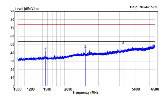
Site : chamber B Condition : Vertical Project Number: 2401U56421E-EM Test Mode : Communication+ Adapter (GQ12-120100-AU) Tester : Dylan
