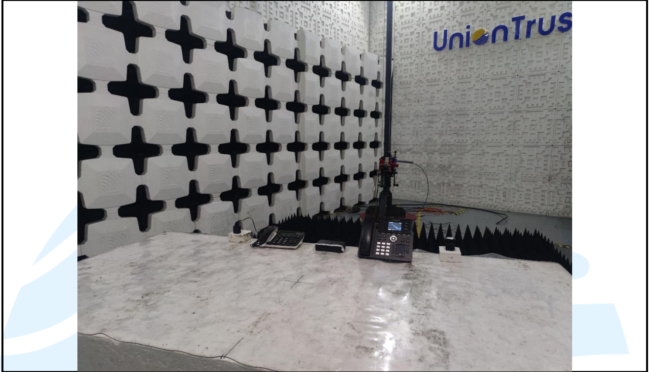
Radiated emission Test Setup-2 (Above 1 GHz)
