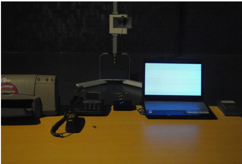
Radiated Emission test view (Above 1GHz)
