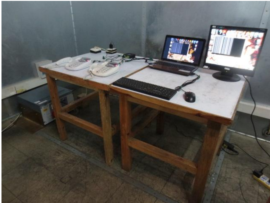
Conducted Emission Test Set-up -Front view
