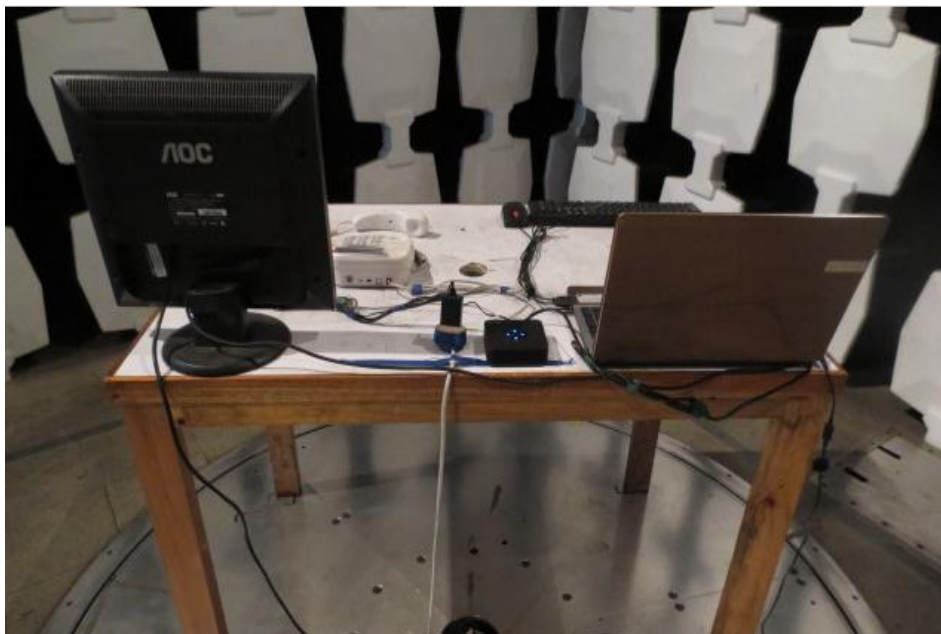
Radiated Emission Test Set-up (Rear View)
