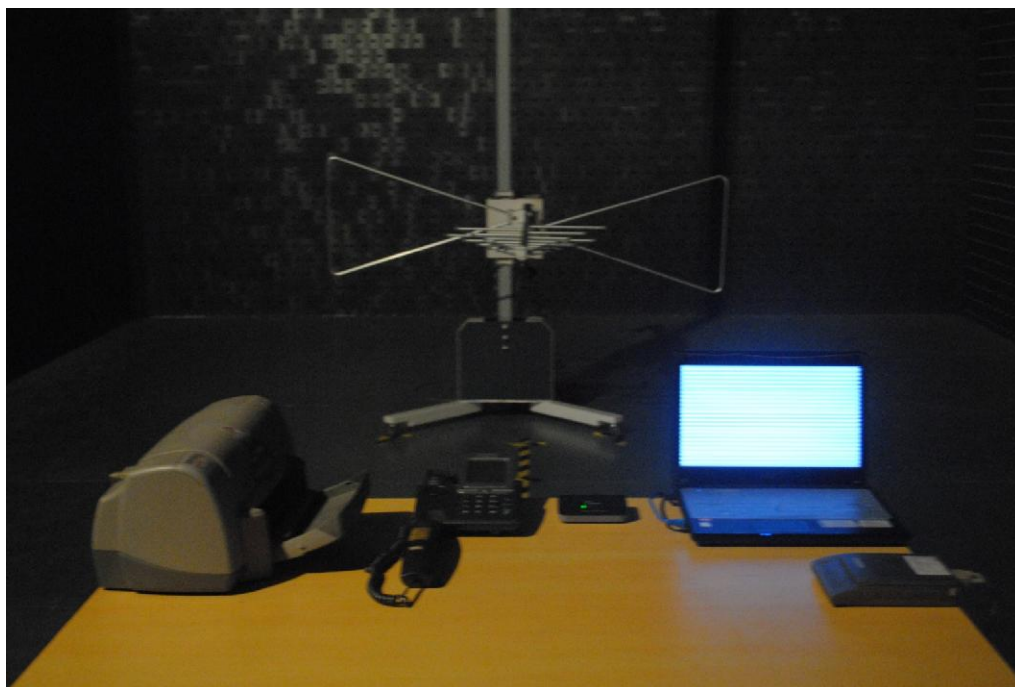
Radiated Emission test view (Frequency above 1GHz)
