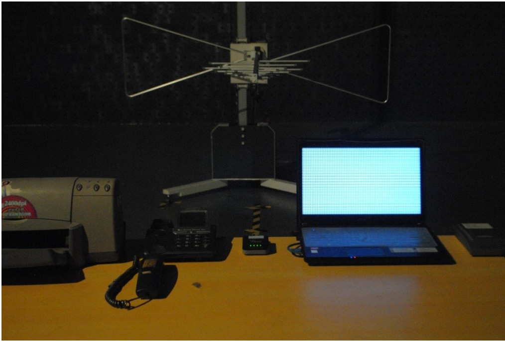
Test Setup Photos YZZHT701V21 Radiated Emission test view (From 30MHz to 1GHz)
