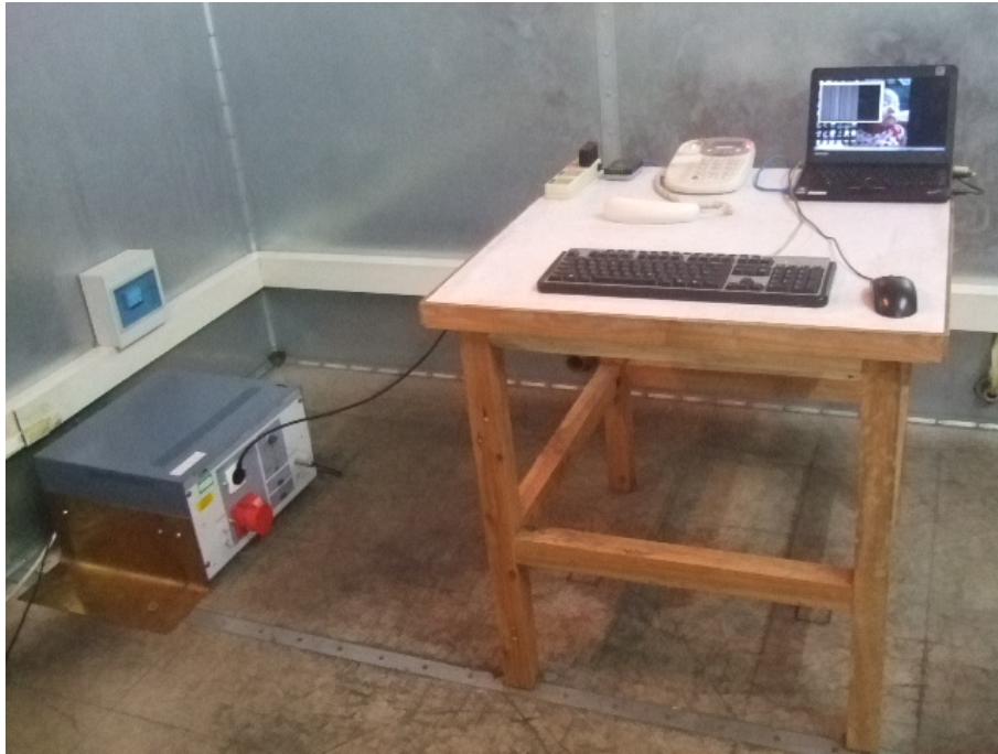
Conducted emission test set-up-front view
