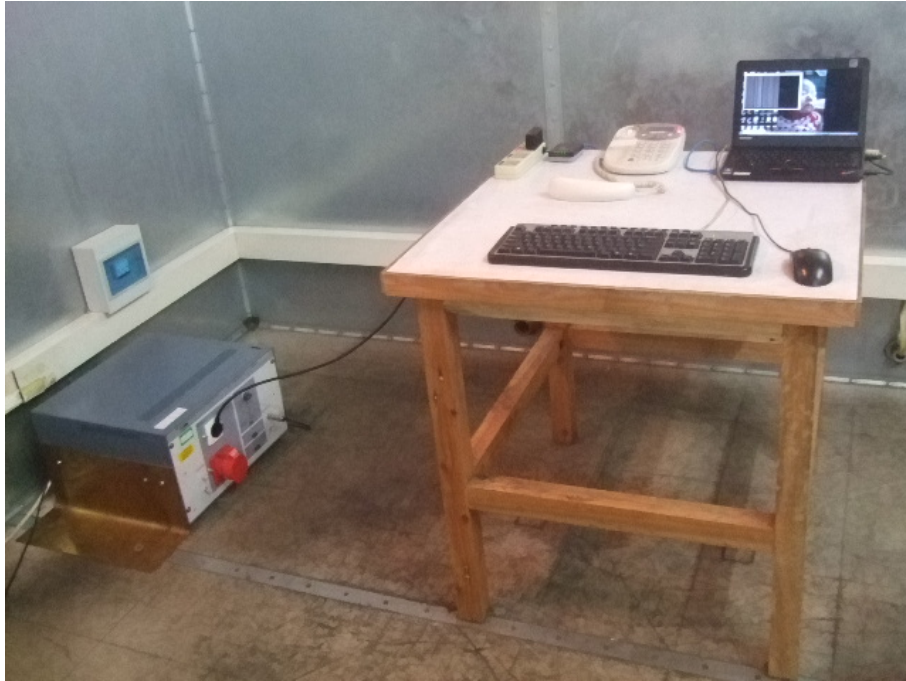
Conducted Emission Test Set-up-Front View
