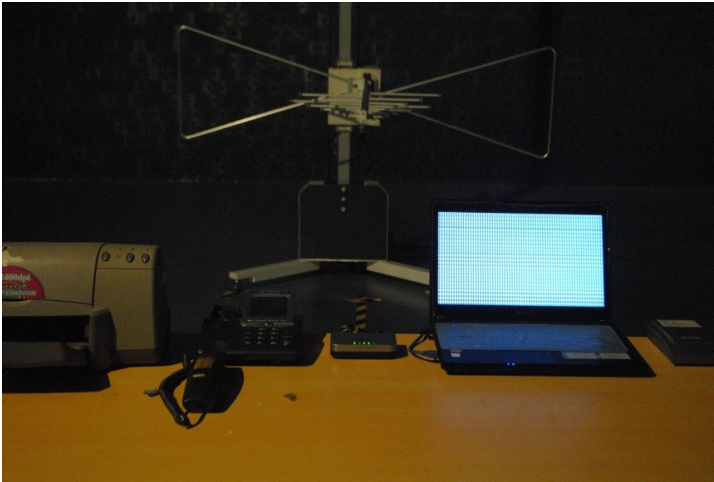
Radiated Emission test view (Frequency above 1GHz)
