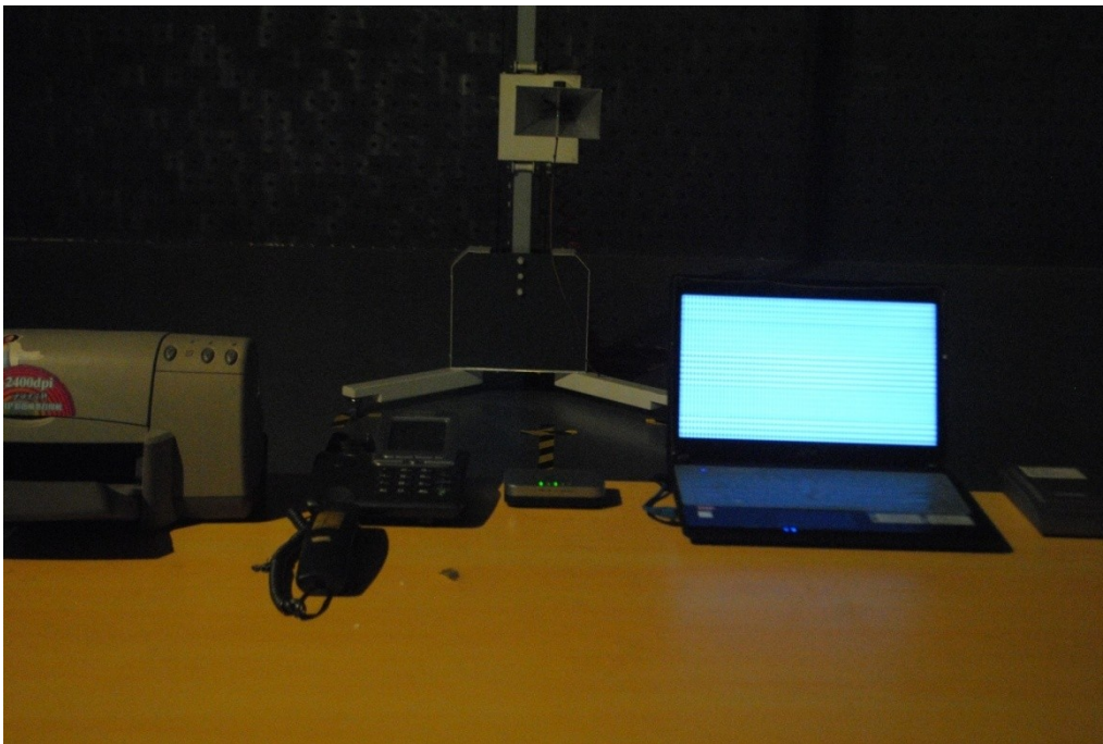
Radiated Emission test view (Frequency above 1GHz)
