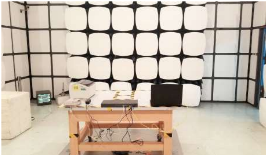
Radiated Emission Test Set-up Rear view (30-1000MHz)
