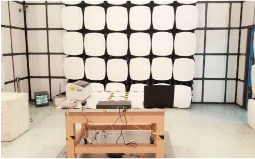
Radiated Emission Test Set-up-Rear View
