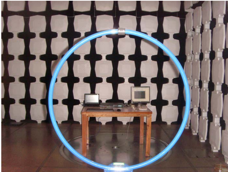
Radiated Emission Test Set-up (9KHz-30MHz)
