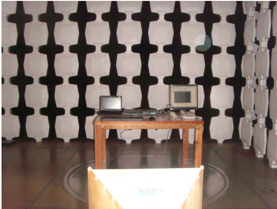
Radiated Emission Test Set-up (Above 1GHz)
