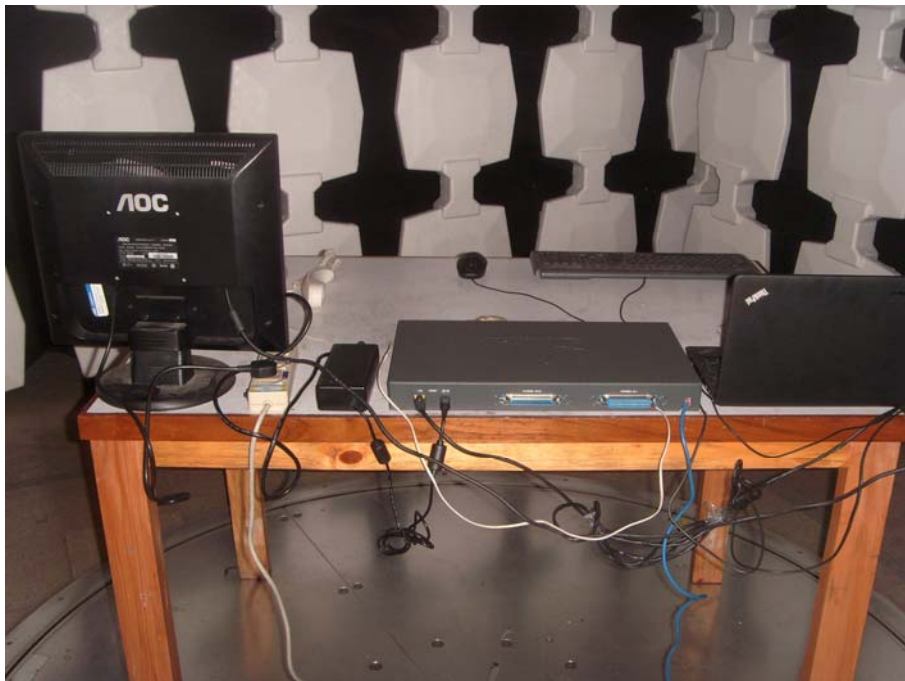
Radiated Emission Test Set-up (rear view)
