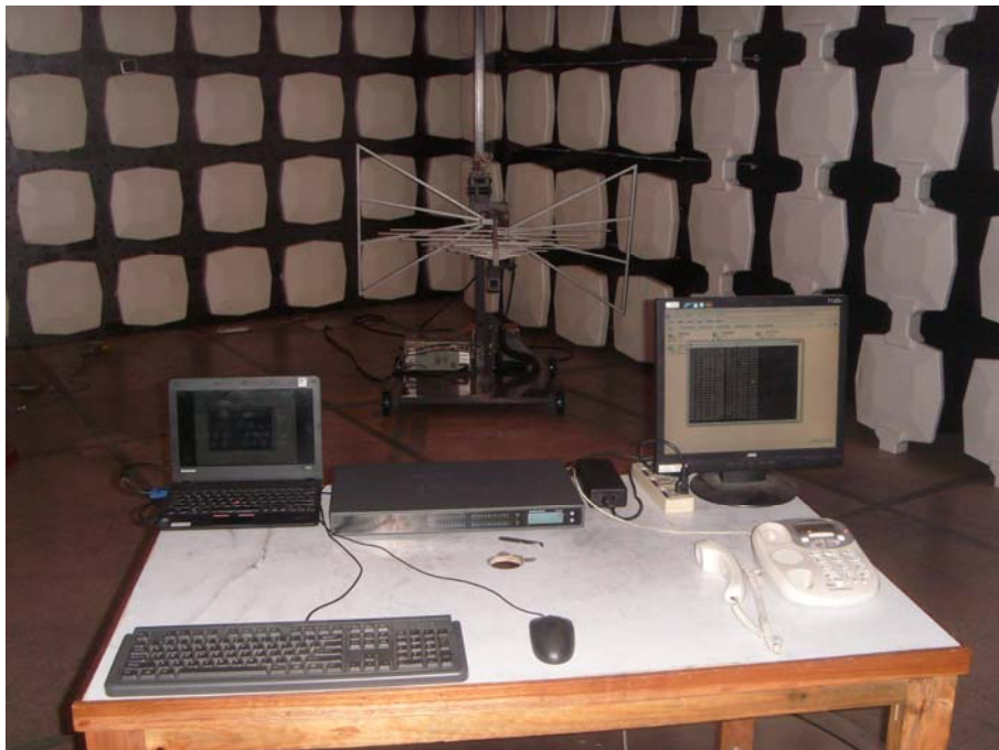
Radiated Emission Test Set-up (Below 1GHz)
