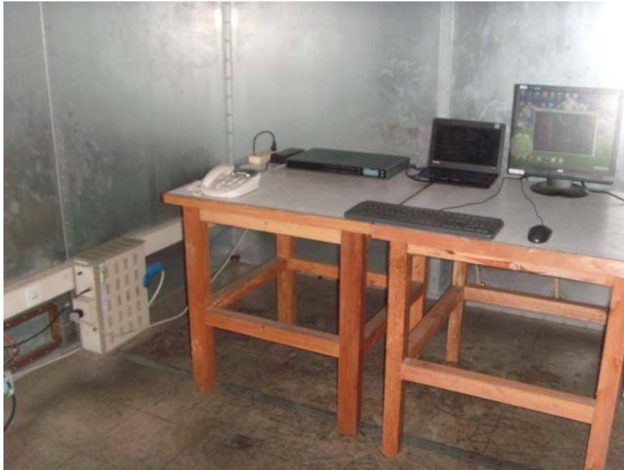
Conducted Emission Test Set-up -front view
