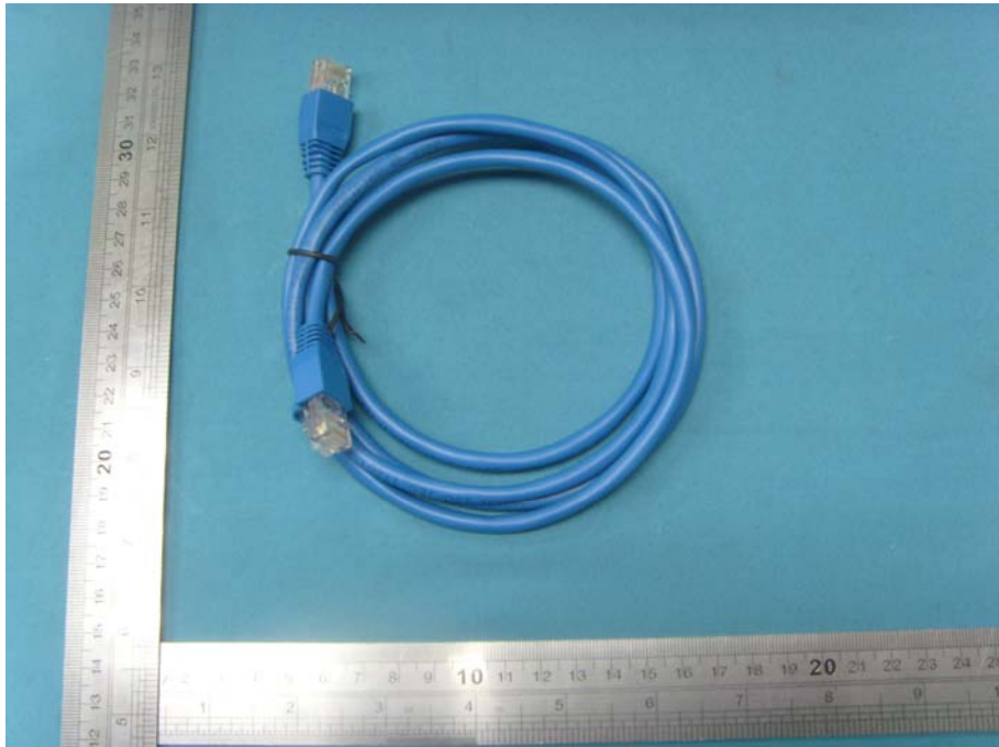
RJ-45 Cable View
