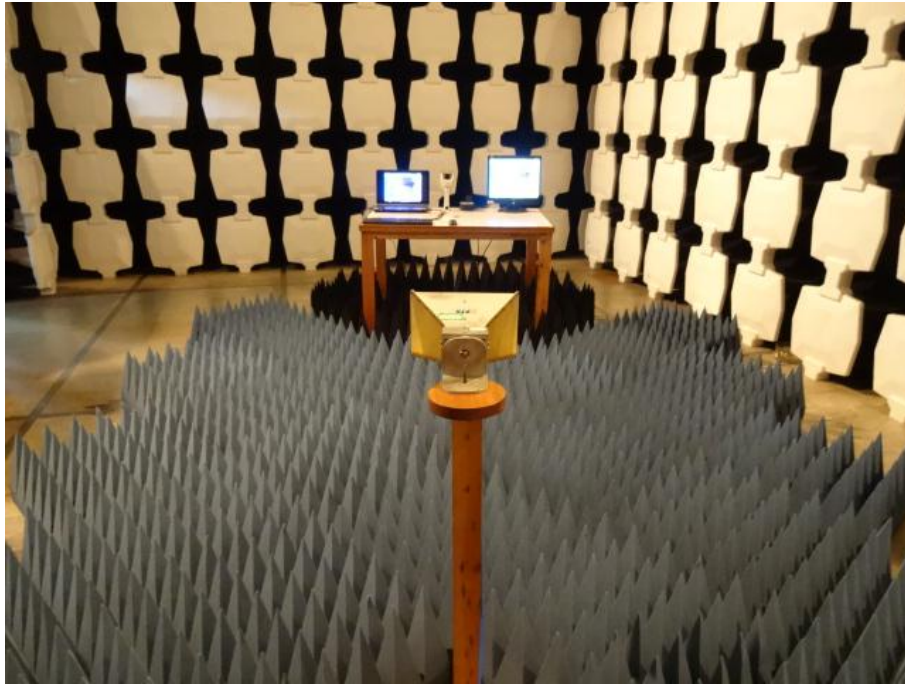
Radiated Emission Test Set-up(Above 1GHz)
