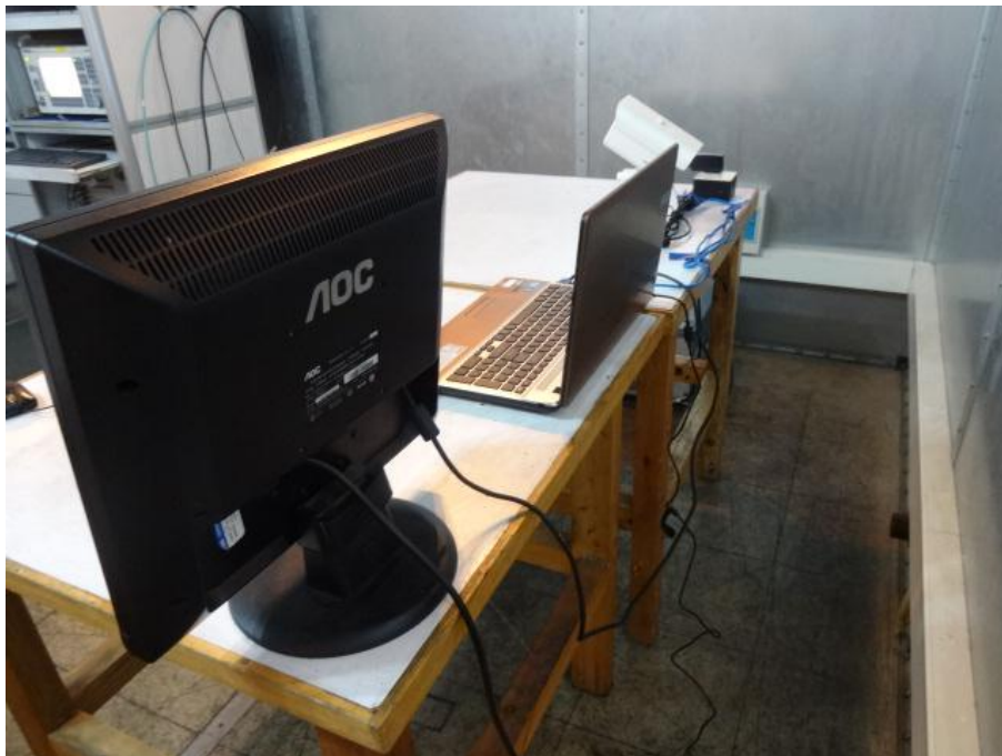
Conducted Emission Test Set-up -Rear view
