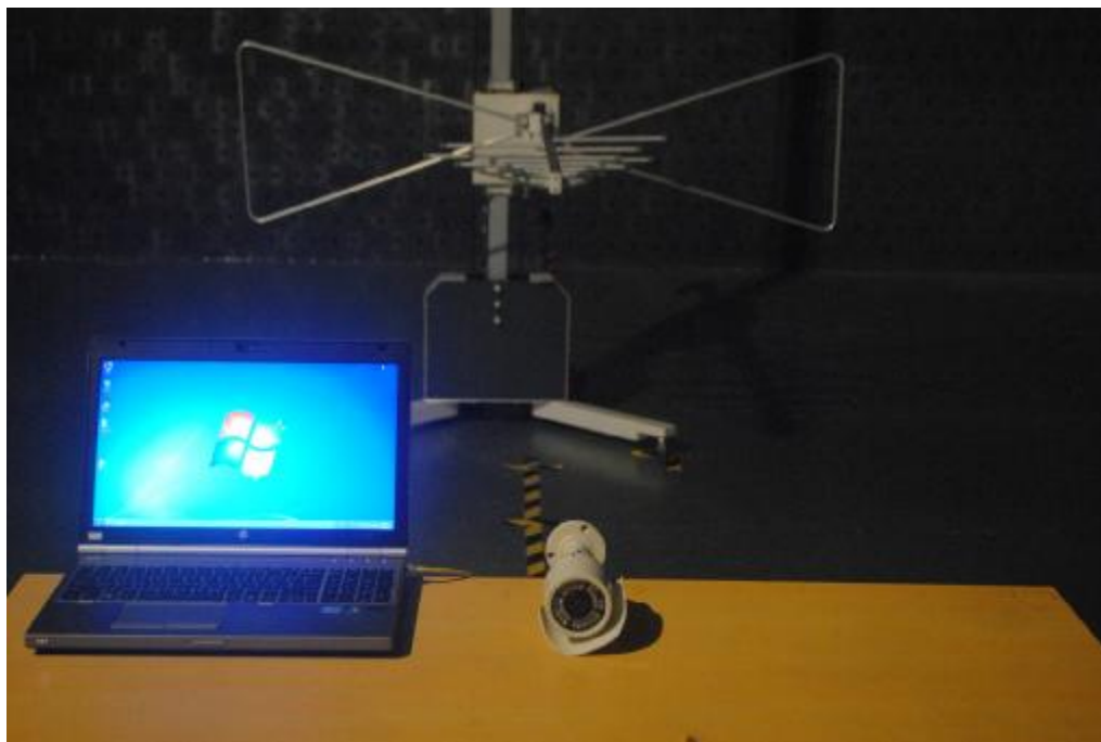
Radiated emission test view
