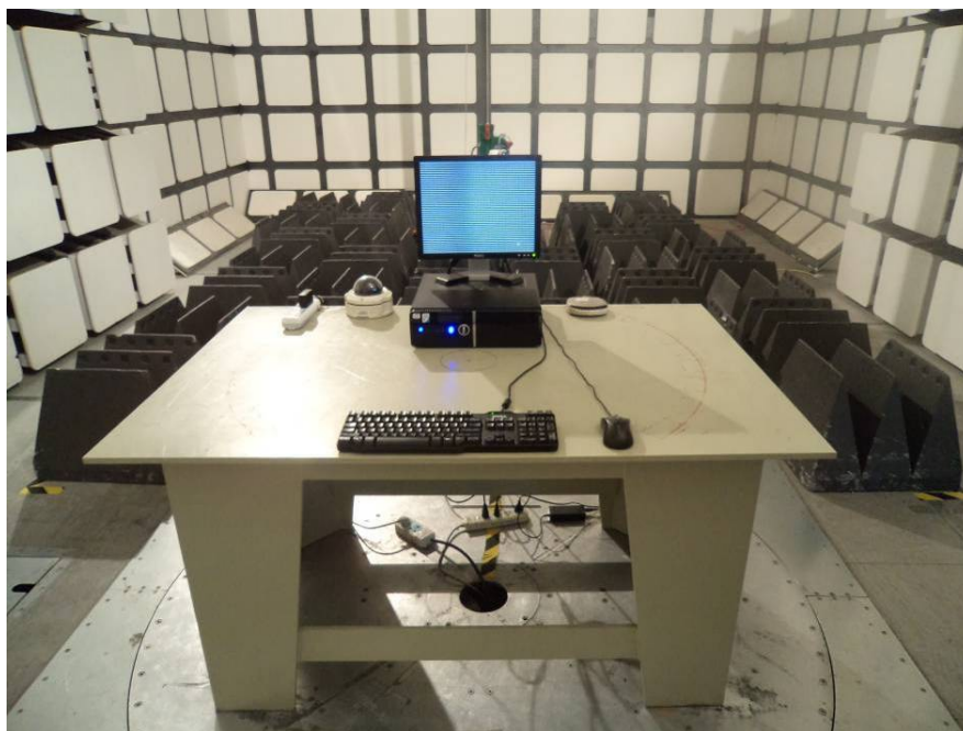
Radiated Emissions - Front View (Powered by AC adapter)
