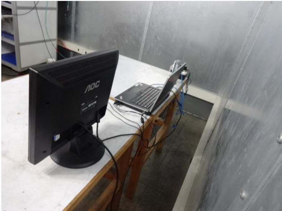
Conducted Emission Test Set-up-Rear View
