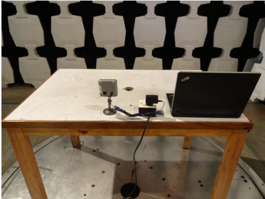
Radiated Emission Test Set-up (Rear View)
