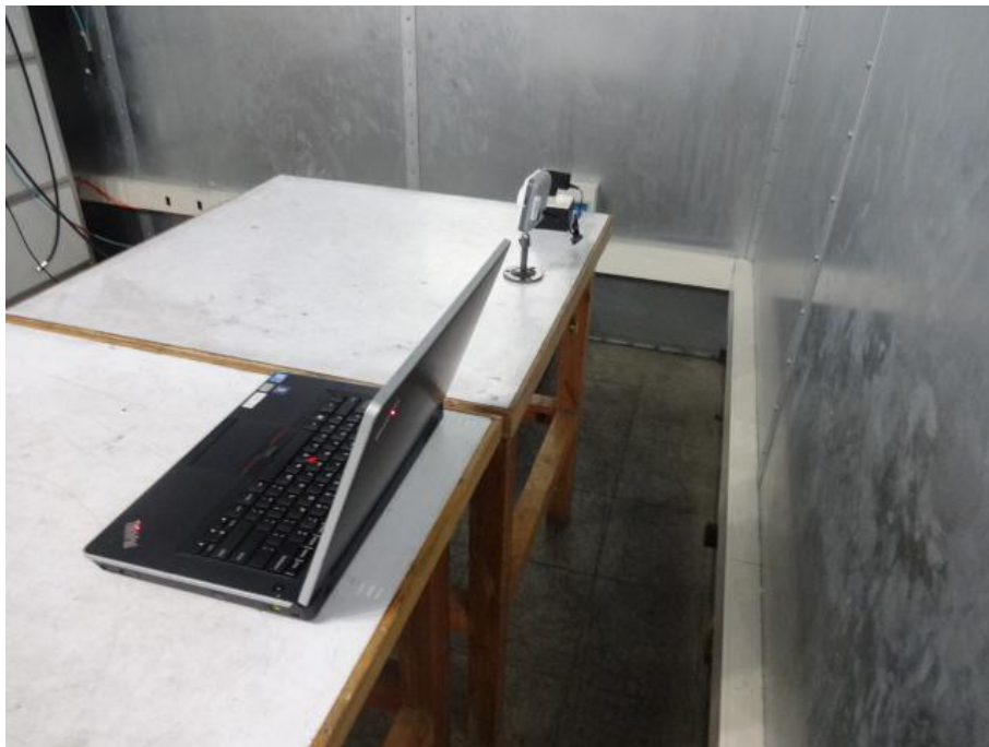
Conducted Emission Test Set-up-Rear View
