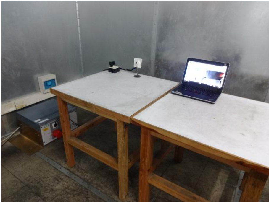
Conducted Emission Test Set-up -Front View
