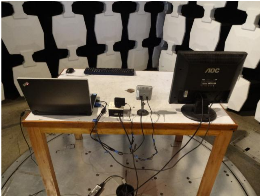
Radiated Emission Test Set-up (Rear View)
