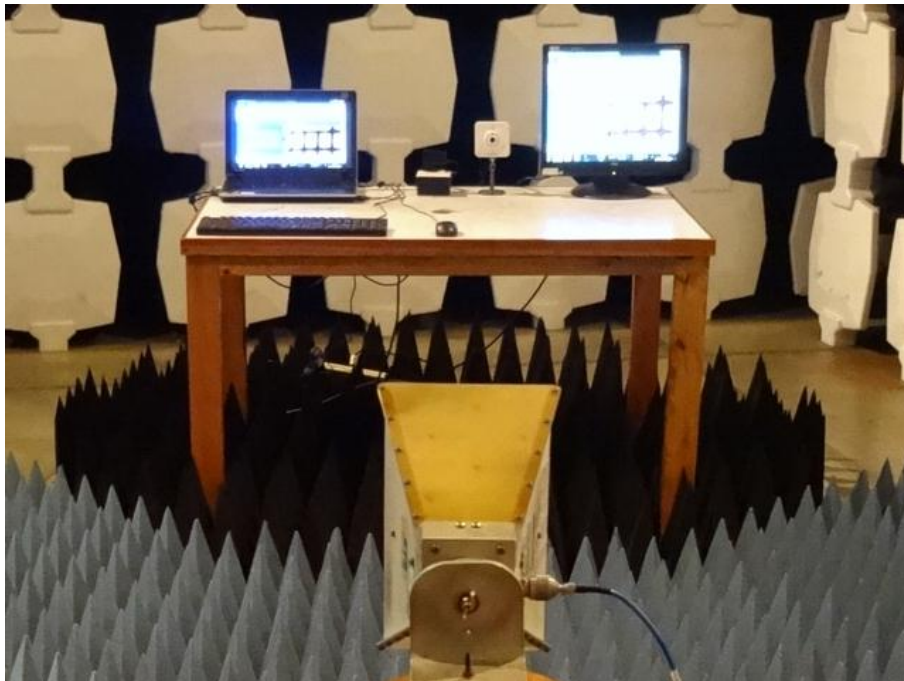
Radiated Emission Test Set-up (Above 1GHz)
