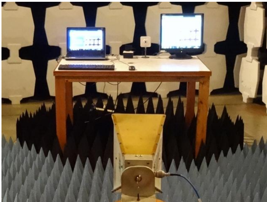
Radiated Emission Test Set-up (Above 1GHz)
