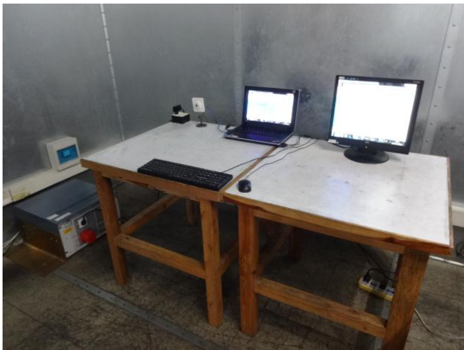
Conducted Emission Test Set-up-Front View
