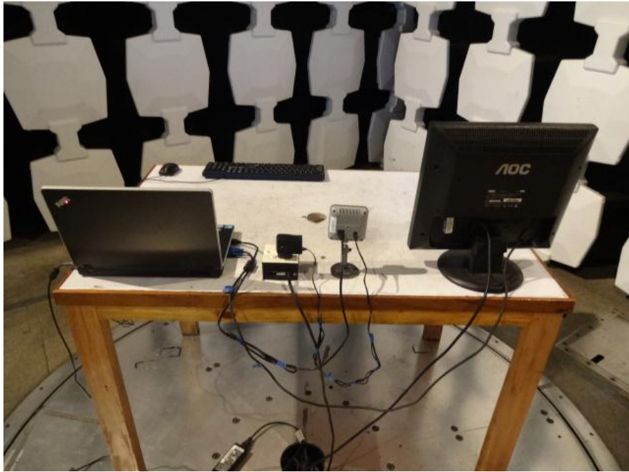
Radiated Emission Test Set-up (Rear View)
