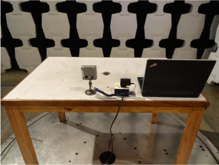
Radiated Emission Test Set-up (Rear View)
