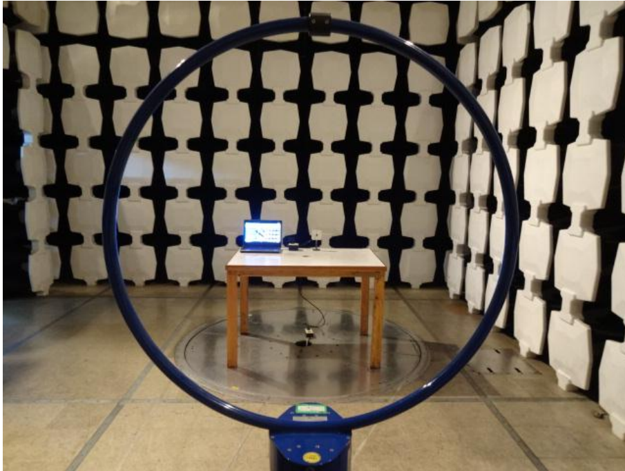
Radiated Emission Test Set-up (9KHz-30MHz)
