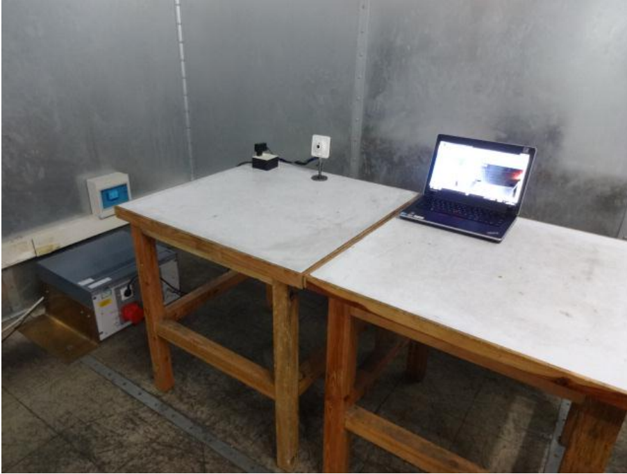
Conducted Emission Test Set-up –Front View
