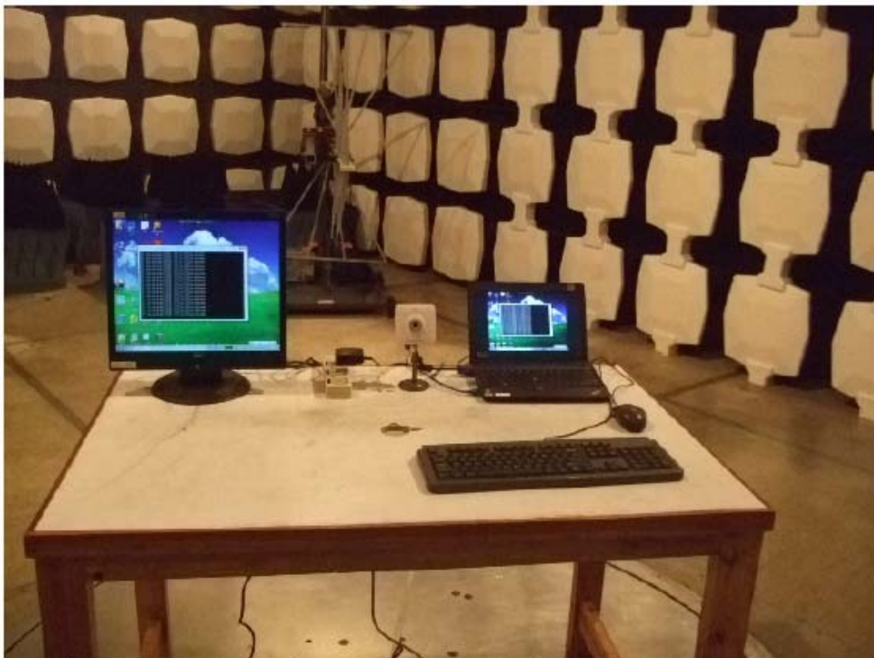
Radiated Emission Test Set-up -below 1GHz
