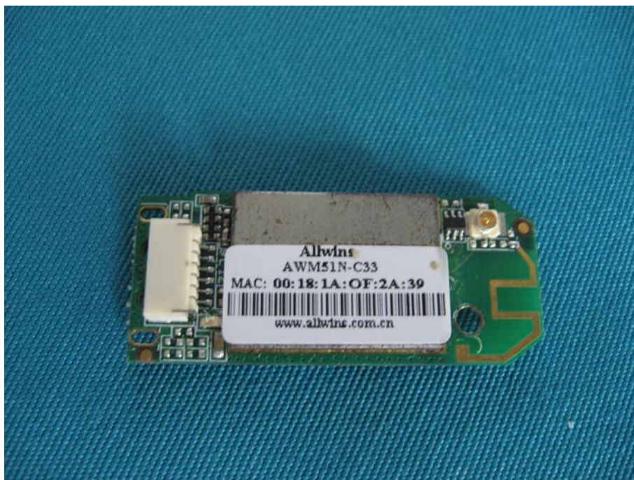
802.11b/g/n module- Front View
