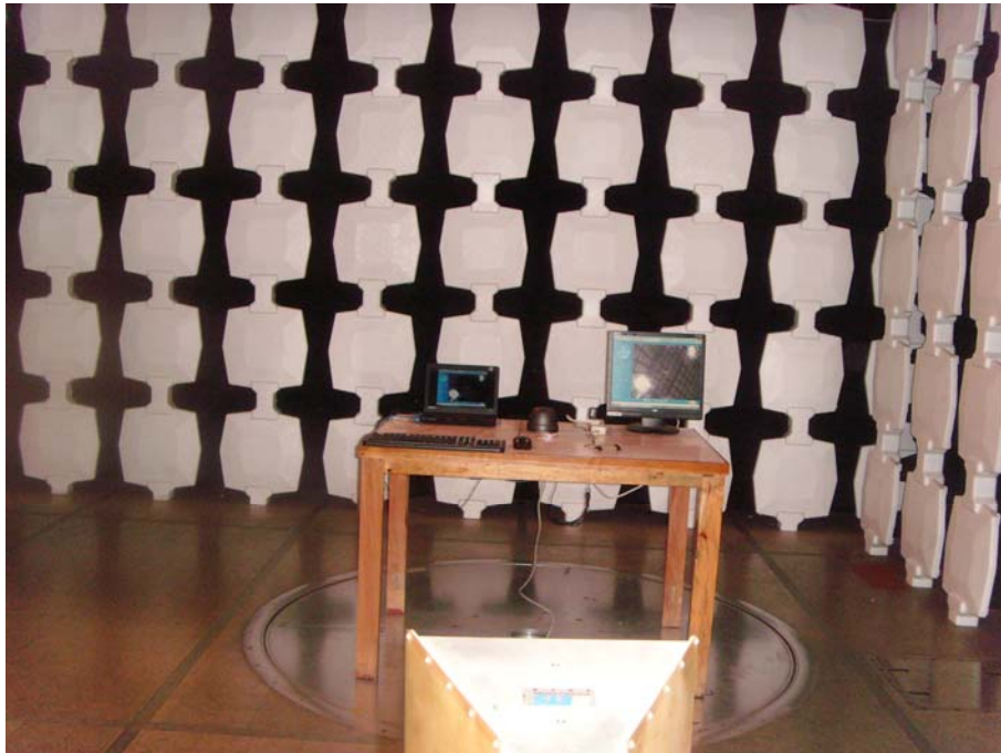
Radiated Emission Test Set-up(Above 1GHz)
