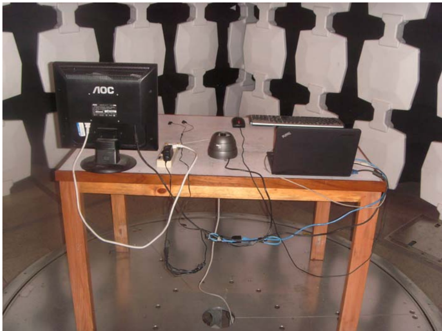
Radiated Emission Test Set-up (Rear view)
