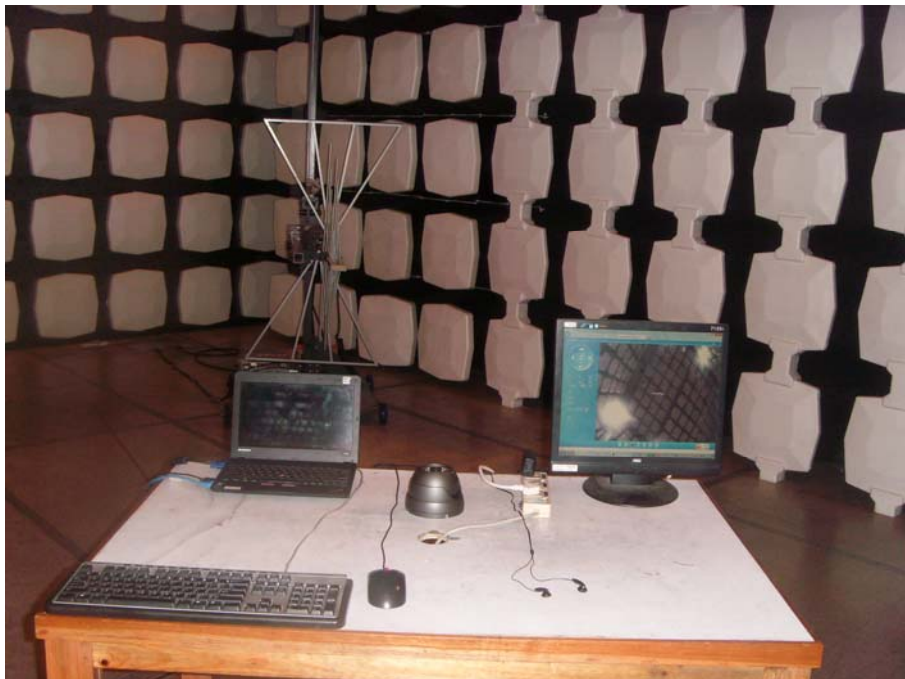
Radiated Emission Test Set-up(Below 1GHz)
