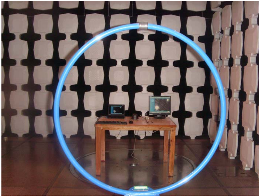
Radiated Emission Test Set-up(9KHz-30MHz)
