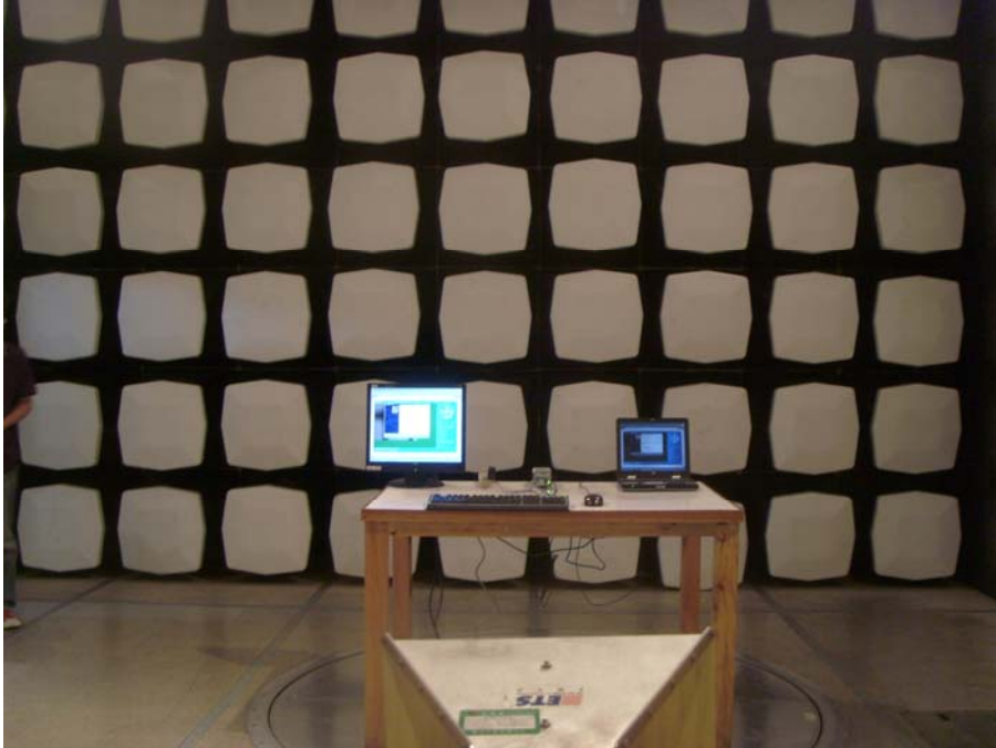
Radiated Emission Test Set-up(Above 1GHz)
