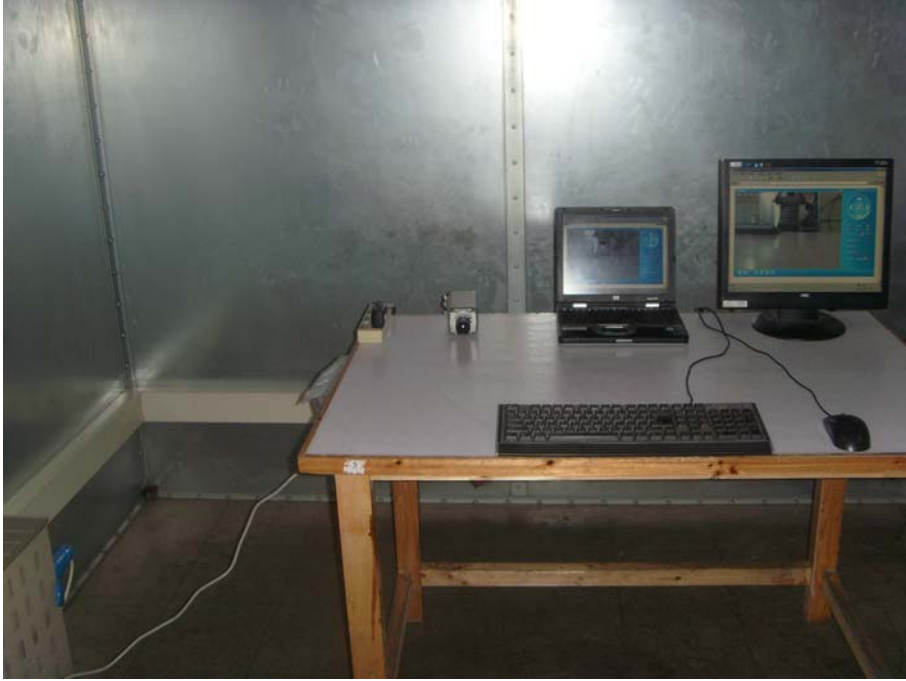
Conducted Emission Test Set-up
