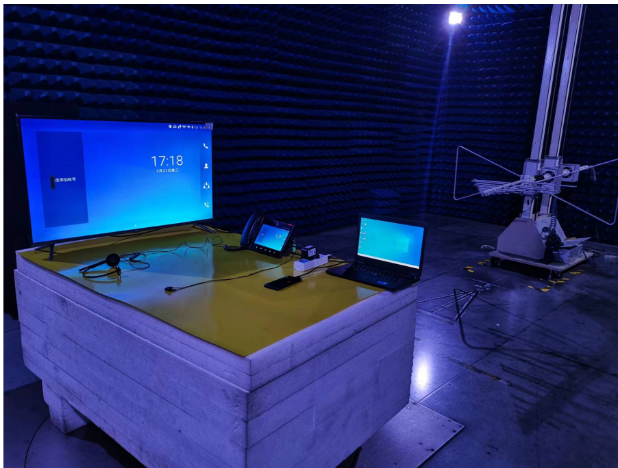
Photo of Radiated Emission Measurement (Below 1G) Powered by Adapter
