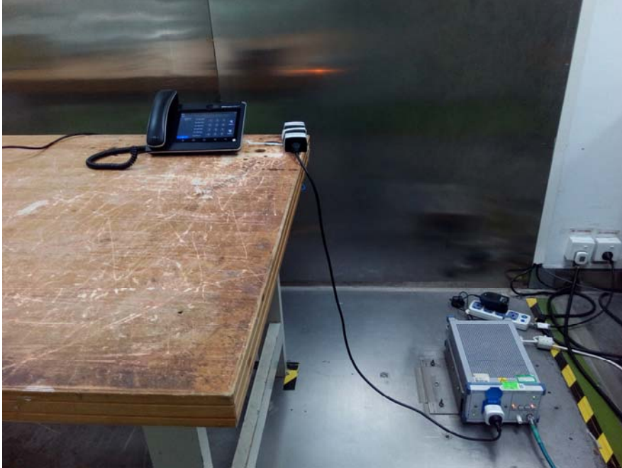
Conducted Emissions - Front View (Powered by POE)
