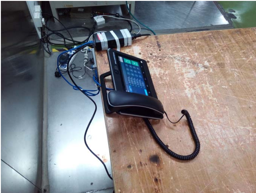
Conducted Emissions - Side View (Powered by POE)
