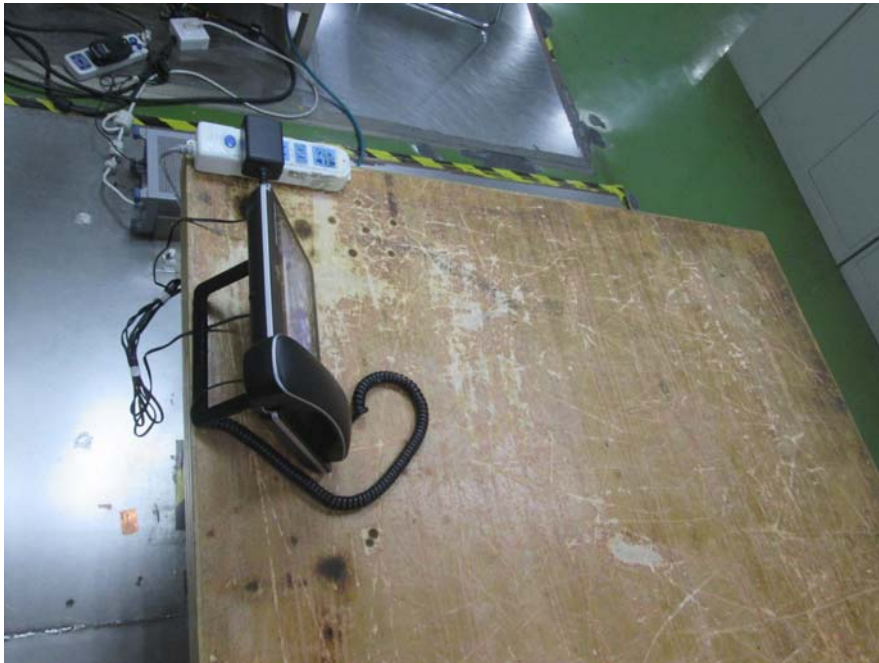
Conducted Emissions - Side View (Powered by Adapter 1)
