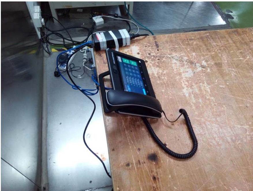
Conducted Emissions - Side View (Powered by POE)
