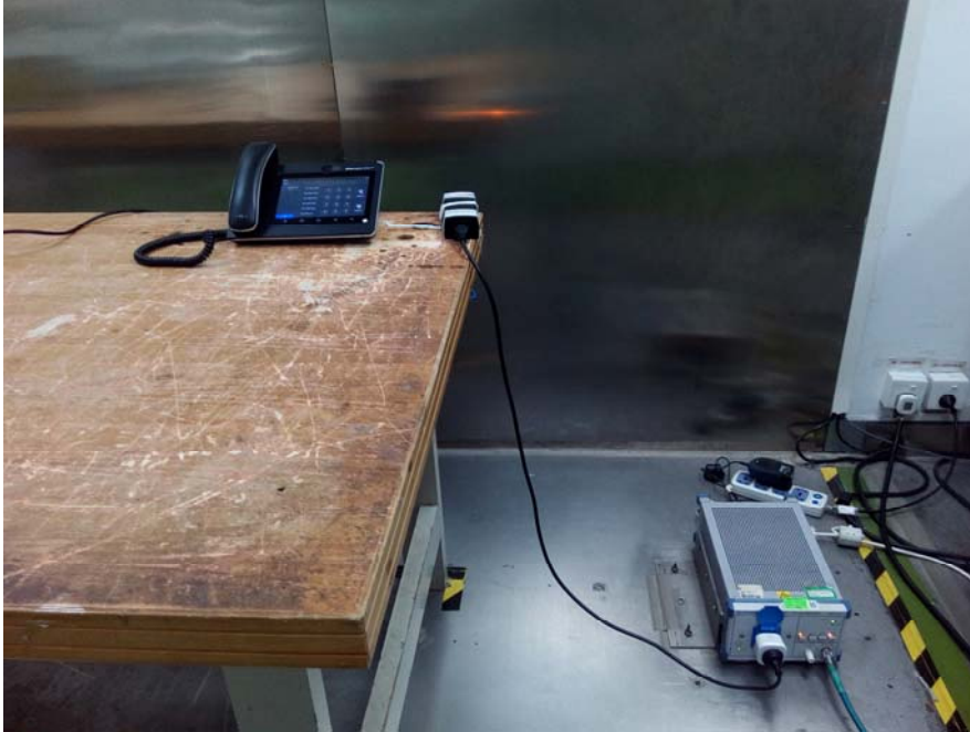
Conducted Emissions - Front View (Powered by POE)
