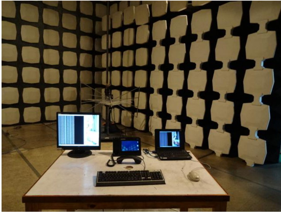
Radiated Emission Test Set-up (Below 1GHz)
